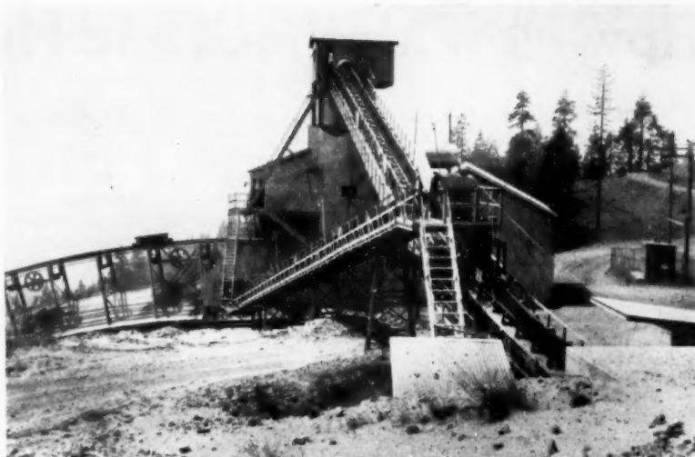
LOADING TERMINAL for the aerial tramway contains a 100-ton surge bin. Ore from screening plant surge pile comes on conveyor belt out of concrete tunnel.
